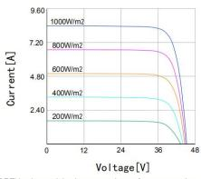
SUNWORTH solar modules have superior performance under low solar irradiation condition ( 200W/  $\rm m^2$  (AM1.5, 25  $^{\circ}C)$
